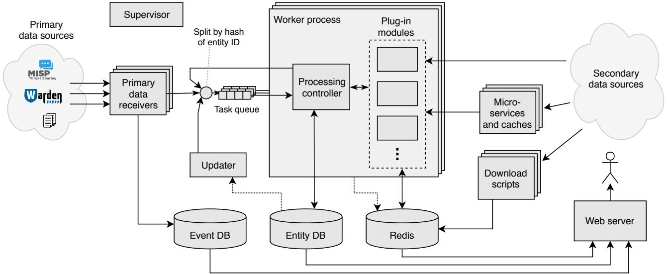
**Figure 1: Architecture of the NERD system**
